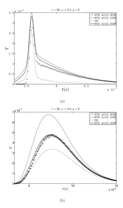
Figure 5: Time history of the dimensionless transmittance: comparison between the RTE solution estimated with MCM (reference solution), the RTE with DOM, the DE and the HTD models for an optical thickness  $\tau = k_a + k_s = 20$ , an albedo  $\omega = 0.5$  (a) and 0.9 (b), and an isotropic phase function.
