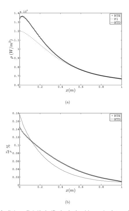
Figure 3: Irradiation profile inside the 1D solar absorber: (a) comparison between the RTE model estimated with MCM (reference solution), P1 and HTD models for an optical thickness  $\tau = k_a + k_s = 4$ , an albedo  $\omega = 0.5$  and a diffuse sphere phase function. (b) Statistical error related to RTE and HTD simulations
