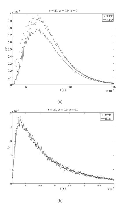
Figure 8: Statistical uncertainties of the MCM solutions obtained by the RTE and by the HTD model for an optical thickness  $\tau = k_a + k_s = 20$ , an albedo  $\omega = 0.9$ , and an isotropic phase function (a) or a Henyey-Greenstein phase function with g = 0.9 (b).
