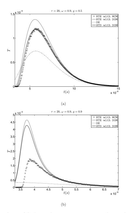
Figure 6: Time history of the dimensionless transmittance: comparison between the RTE model estimated with MCM (reference solution), the RTE with DOM, the DE and the HTD models for an optical thickness  $\tau = k_a + k_s = 20$ , an albedo  $\omega = 0.9$ , and a Henyey-Greenstein phase function with g = 0.5 (a) and with g = 0.9 (b).
