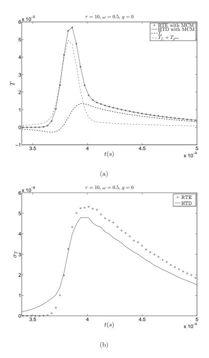
Figure 7: MCM solutions of the RTE and the HTD models. Time history of the dimensionless transmittance (a), and of the statistical uncertainties (b) for an optical thickness  $\tau = k_a + k_s = 10$ , an albedo  $\omega = 0.5$ , and an isotropic phase function.
