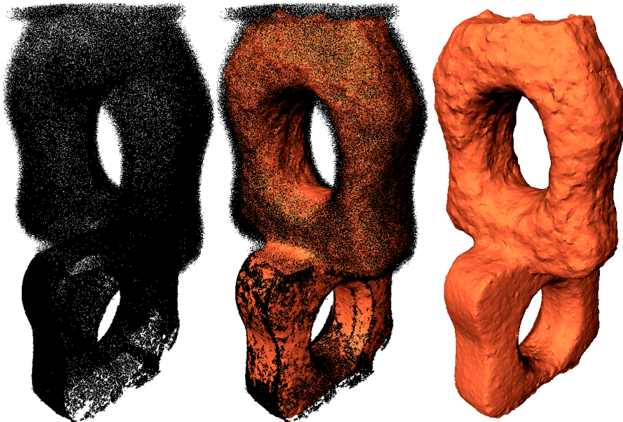
FIGURE 7. Two levels of noise . Left: raw point set with additional noise on the top half part. Middle: point set & reconstruction. Right: reconstruction only (running time: 242s).
