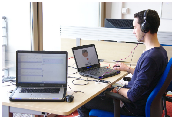
Figure 5: Our experimental setup. A BVP sensor connects subject’s earlobe to the first laptop, where the human-agent interaction takes place. Subject is wearing a headset to listen to the speech synthesis. A second laptop is used by the experimenter to monitor heartbeats detection.
