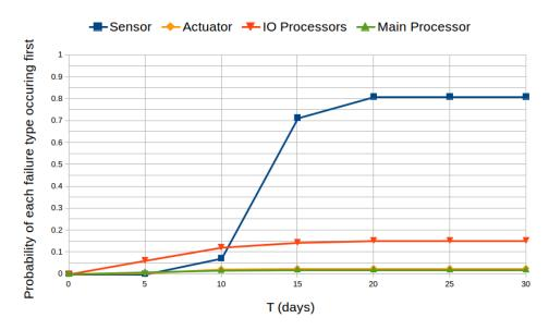
Figure 4: The probability that each of the 4 failure types is the cause of system shutdown in the first T time of operation
