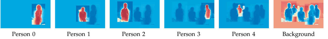
Fig. 3: Illustration of the occlusion-based unary costs for the example in Figure 1. From left to right we show the unary costs for persons labelled 0 – 4 and the background. The cost for a pixel to take a label (person or background) is denoted by the red (low) - blue (high) spectrum of colours. Here we observe the effect of accumulating the label likelihoods in a front-to-back order. For example, in the illustration for Person 4, a low cost (red) for taking label 4 is observed only for the pixels that are not occluded by the other people in front. ( Best viewed in colour. )
