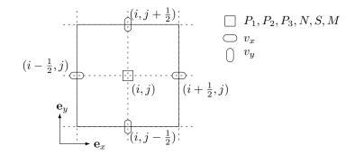
Figure 3. Discretization of unknown variables on one cell grid.
