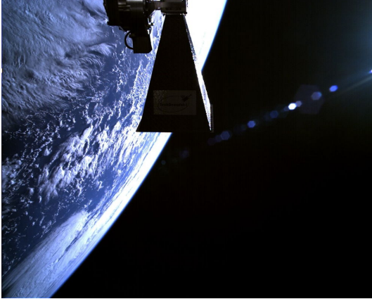
Fig. 20: Supervision Camera. Image from camera on TDS-1 of APM with Earth in the background.
