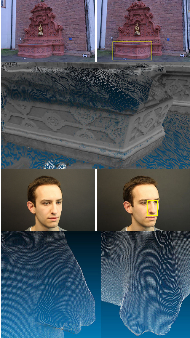
Figure 1. Closeups on reconstruction results obtained using classical variational matching across a pair of views. The Fountain-P11 [5] (top) and our face1 data set (bottom). Please note, the deterioration along the rim of the fountain and the tip of the nose.
