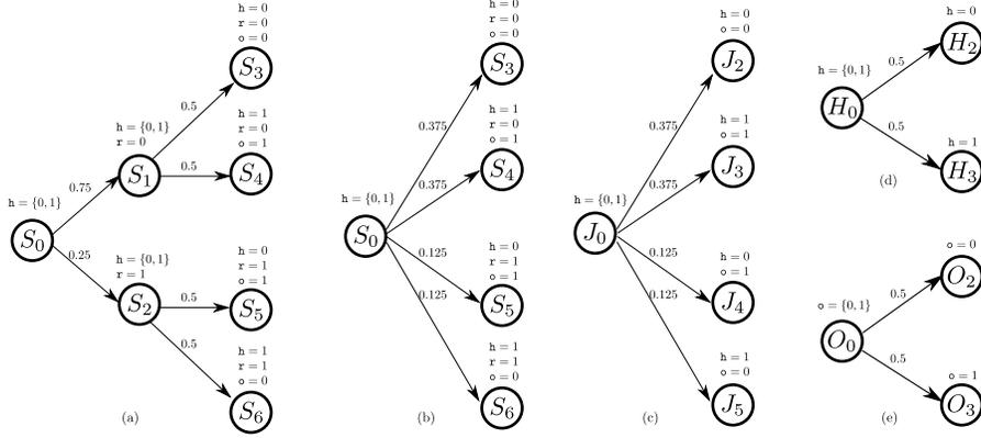
Fig. 1: Bit XOR example: a) Markov chain semantics  $\mathcal{C}$ . b) Observable reduction  $\mathcal{C}$ . c) Joint quotient  $\mathcal{C}|_{(o,h)}$ . d) Secret's quotient  $\mathcal{C}|_h$ . e) Observer's quotient  $\mathcal{C}|_o$ .
