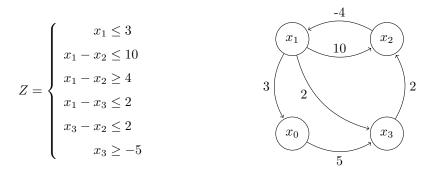
Figure 7. Graph representation of extended clock constraint.
