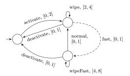
Fig. 5 Weighted modal transition system modeling a simple wiper control component of a car.
