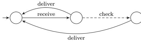
**Fig. 1** Modal transition system modeling a simple email system, with an optional behavior: Once an email is received it may *e.g.* be scanned for containing viruses, or automatically decrypted, before it is delivered to the receiver.
