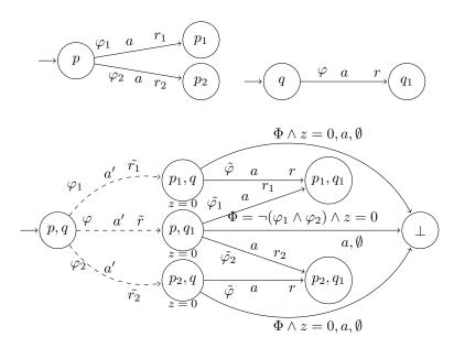
Figure 13.: A timed game constructed for bisimilarity checking of two simple timed automata
