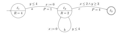
Figure 9.: A weighted timed automaton with two clocks.
