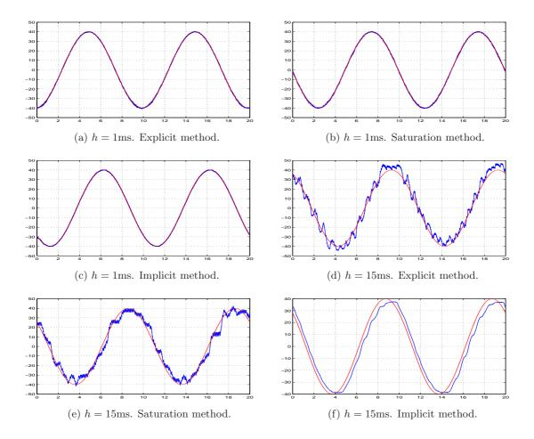
Figure 2: Real position y (mm) in blue and  $y_d$  (mm) in red, under h=1ms and h=15ms for  $G=10^4$ . Real position y in blue and  $y_d$  in red.
