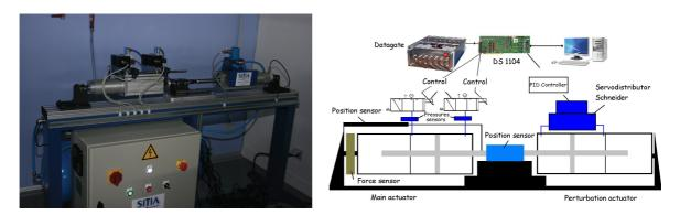
Figure 1: [18] Photography and scheme of the electropneumatic system.
