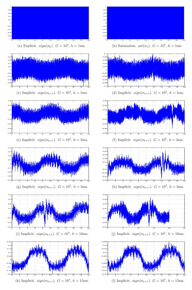
Figure 4: Switching function: Comparison between explicit method  $(sign(s_k))$ , saturation method  $(sat(s_k))$  and implicit method  $(sign(s_{k+1}))$ .
