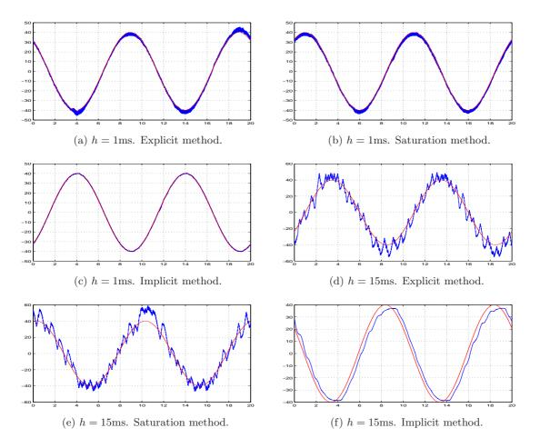
Figure 3: Real position y (mm) in blue and  $y_d$  (mm) in red, under h=1 ms and h=15 ms for  $G=10^5$ .
