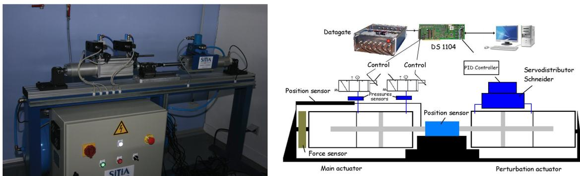
Figure 1: [18] Photography and scheme of the electropneumatic system.
