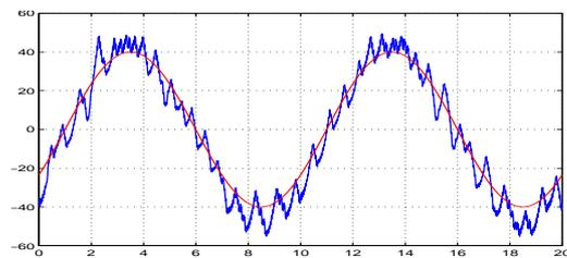
(d)  $h = 15\text{ms}$ . Explicit method.
