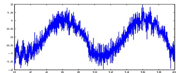
(l) Implicit Method.  $G = 10^5$ ,  $h = 15\text{ms}$ .Figure 5: Comparison of control  $u$  between explicit method, saturation method and implicit method.
