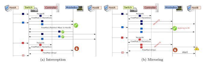
Figure 4: SDN support for Middlebox-based analysis
