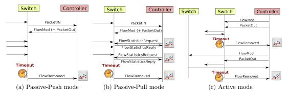
Figure 3: OpenFlow-based monitoring
