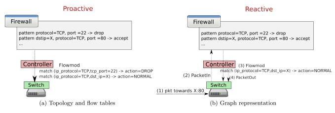
Figure 2: OpenFlow-based stateless firewalls
