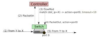
Figure 1: OpenFlow packet processing
