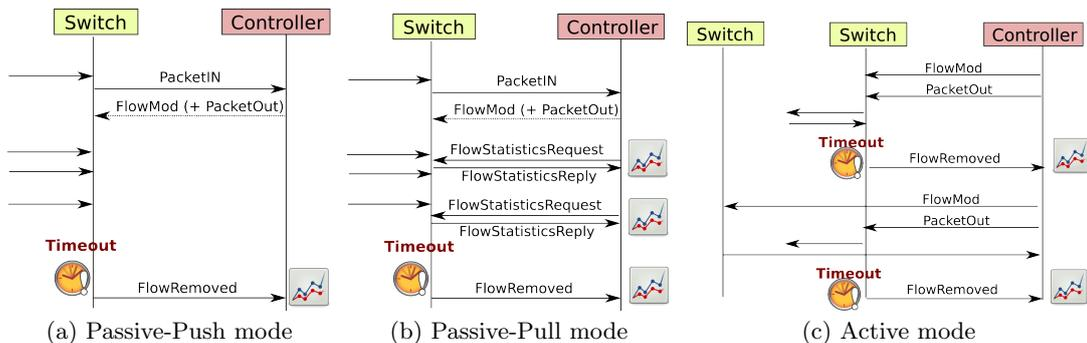
Figure 3: OpenFlow-based monitoring
