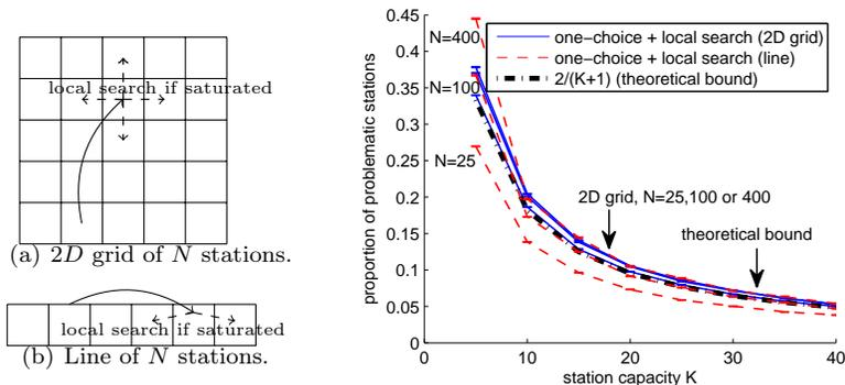
FIGURE 7. Influence of the local search for the one-choice model. Proportion of problematic stations as a function of the station's capacity  $K$  for two geometric models: 2D grid and the line. The parameters are  $s = K/2$  and  $N = 25, 10, 400$ .
