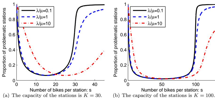
FIGURE 1. Proportion of problematic stations as a function of the number of bikes per station for two values of the size of stations  $K$ . On the  $x$ -axis is the average number of bike per station  $s$ . For both scenarios, we plot  $\lambda/\mu = 0.1$ ,  $\lambda/\mu = 1$  and  $\lambda/\mu = 10$ .
