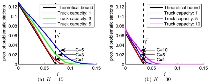
FIGURE 11. Proportion of problematic stations as a function of the redistribution rate  $\gamma/\lambda$ . We compare the theoretical analysis with simulations for various truck capacities. The theoretically optimal redistribution rate is  $\gamma^* = 1/(K - 1)$ .
