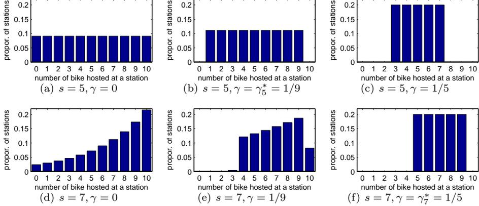
FIGURE 4. Illustration of Theorem 3: distribution of station occupancy. The station capacity is  $K = 10$ . Two fleet sizes  $s = 5$  and  $s = 7$  and three redistribution rates  $\gamma = 0$ ,  $\gamma = 1/9$  and  $\gamma = 1/5$  are compared.
