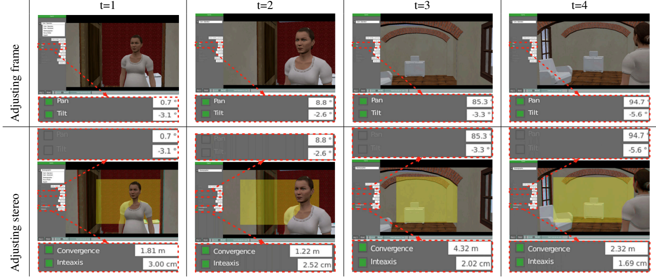
Fig. 2. First row (Adjusting frame): the user in Camera Operator role, controls the frame of the camera interactively, and follows the woman as she enters the room. The parameters of the camera, Pan and Tilt, are recorded (marked with a green box). Second row (Adjusting stereo): once the frame has been recorded, the user switches to Stereographer role and controls the interaxial and convergence distance interactively. The parameters of the camera, Pan and Tilt, are replayed (marked with a gray box) while Convergence and Interaxial are recorded (marked with a green box). The yellow semitransparent rectangle in the images shows the stereoscopic convergence plane in the scene.
