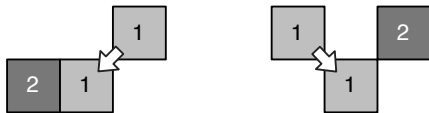
Fig. 2. Minimal 8-connected basic patterns generating temporary labels: stair (left) and concavity (right)
