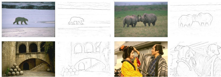
Figure 4.3: Edge detection results obtained with the software package of Xiaofeng and Bo [2012] on the Berkeley segmentation dataset BSD500 [Martin et al., 2001]. Four pairs of images are presented. The left ones represent input images and the right ones confidence maps for the presence of edges. Dark values represent high confidence. Best seen by zooming on a computer screen.
