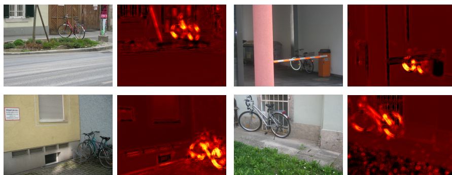
Figure 4.2: Results of pixelwise classification of test images from Mairal et al. [2008a]. Two dictionaries are learned beforehand, one from images containing a bicycle, and one from images corresponding to background only. For each of the four test images displayed here, we also display a confidence map for the presence of a bicycle. For each pixel, a confidence value is computed for a patch centered at the pixel, by comparing the residual of the reconstruction errors obtained with the two dictionaries; yellow bright pixel values represent high confidence, whereas dark red pixel values represent low confidence.
