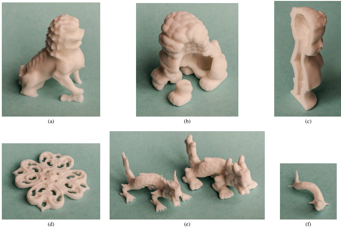
Figure 14: Some 3D printed models obtained by our method. (a) The lion model slightly eroded. (b) The complex CSG intersection and dilation of Figure 13, when considering the truncated cuboctahedron. (c) Section cut of the difference between the original buste model and its erosion. (d) The closing of the filigree model with a cube. (e) The original dragon (left) and the dilated dragon (right) of Figure 12. (f) An eroded dragon.
