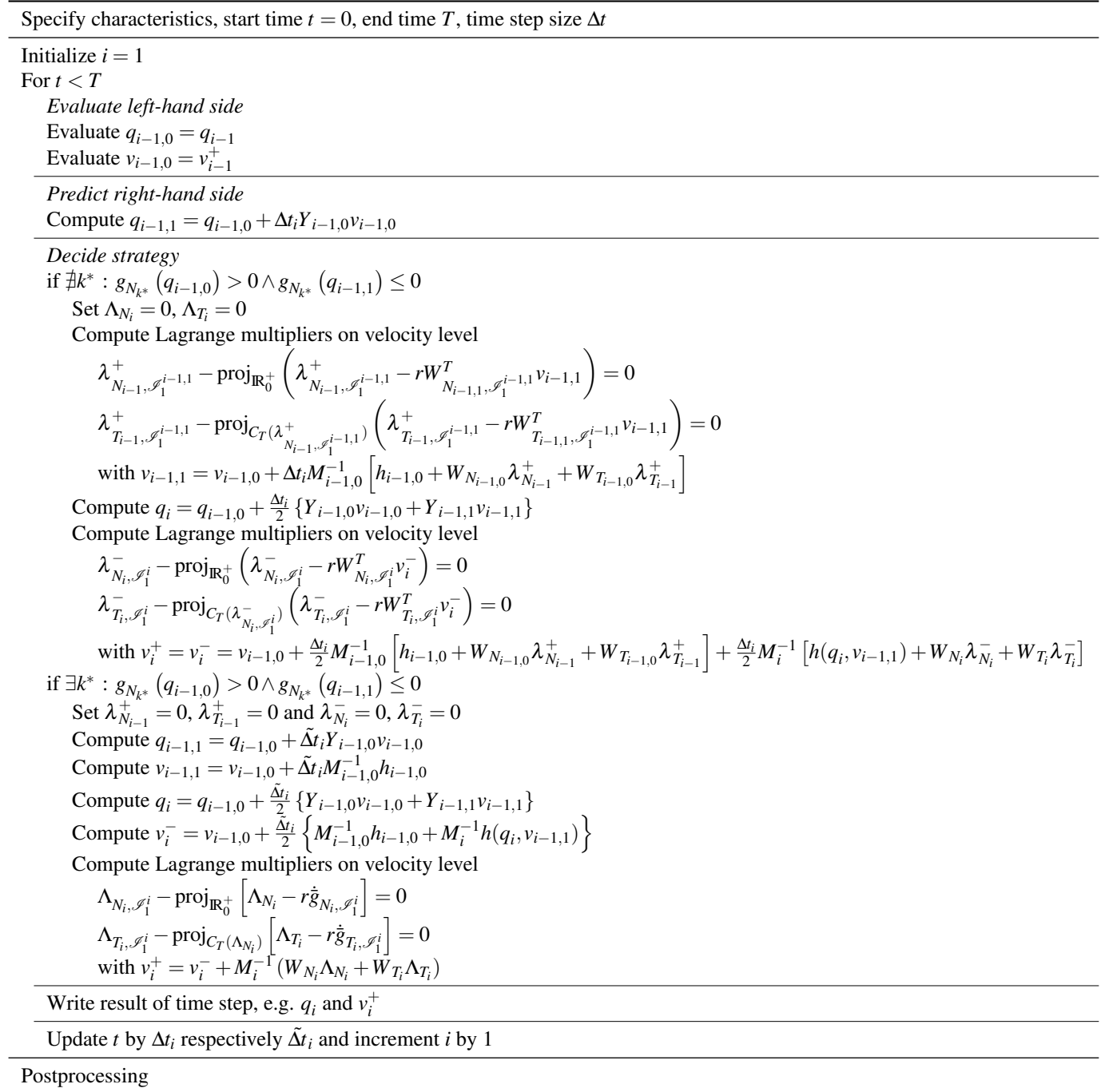
Figure 24: Flowchart of the half-explicit timestepping scheme on velocity level, variant for MBSim.
