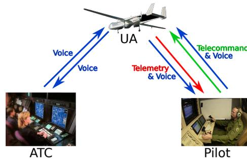
**Fig. 1.** Architecture of an Unmanned Aircraft System.
