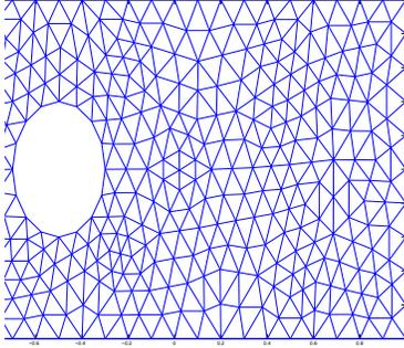
**Figure 1: Triangulation of the domain**  $[-1, 1] \times [-0.5, 0.5] \setminus D((-0.5, 0), 0.2)$ .
