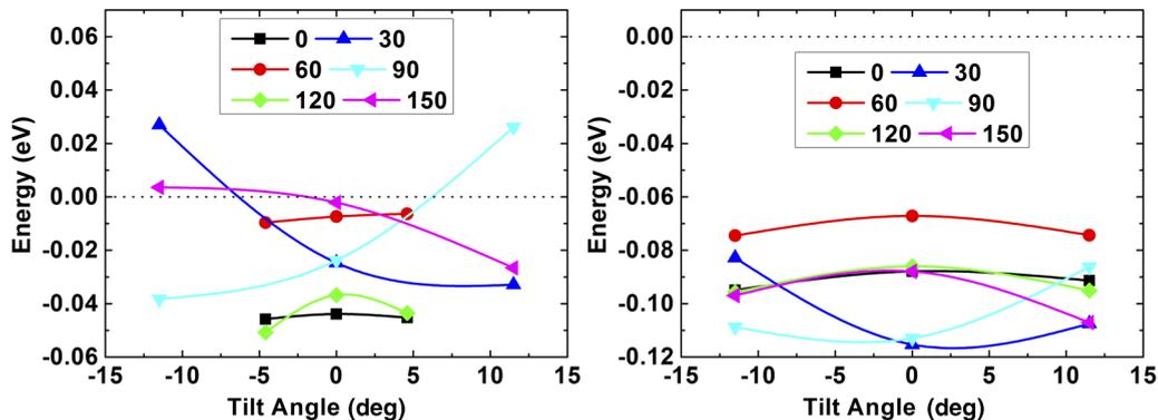
FIG. 6. (Color online) Adsorption energy per  $C_{60}$  vs tilt angle of the right  $C_{60}$  at different rotational angles (see Fig. 5) on (a) Ag(111) and (b) Au(111). The energy scale is relative to the hex-vac + hex-top configuration (dotted horizontal line).
