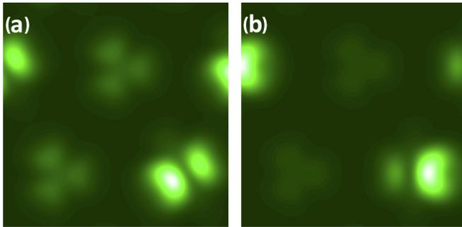
FIG. 7. (Color online) Simulated STM image of the mixed configurations at +1 V for the right C<sub>60</sub> (a) at 120° with tilt angle of 4.6° on Ag(111) and (b) at 90° on Au(111) with tilt angle of -11.5° (see Fig. 5).
