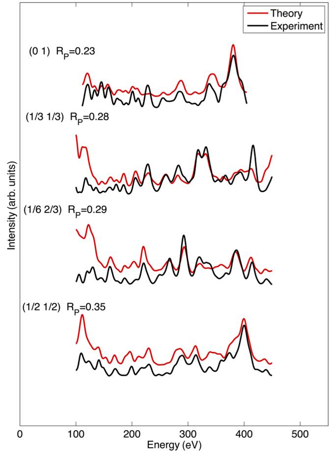
FIG. 4. (Color online) Representative LEED spectra from the best-fit mixture of 80% hex-par vac and 20% 6:6 C-C top for C<sub>60</sub> on Au(111). The full data set is provided in Ref [37].
