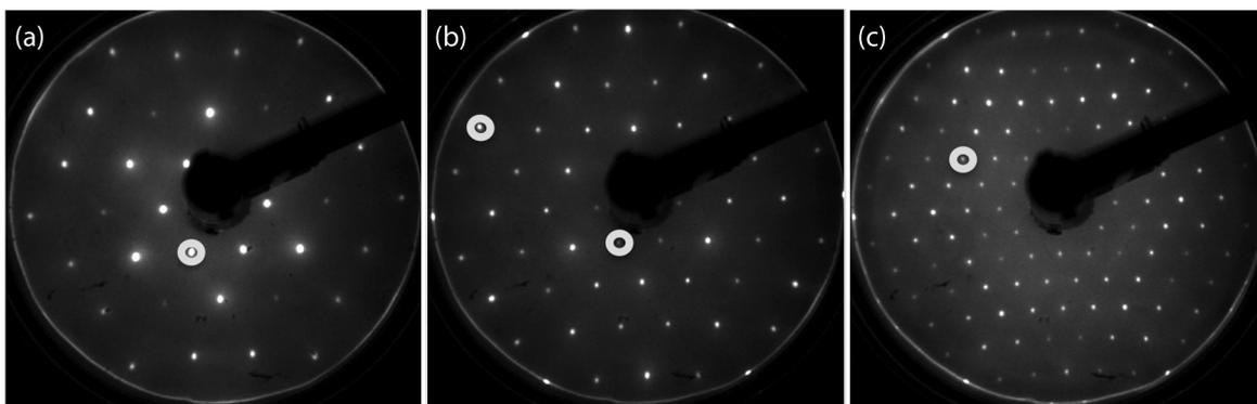
FIG. 3. LEED patterns from the Au(111)- $(2\sqrt{3} \times 2\sqrt{3})R30^\circ$ -C<sub>60</sub> structure at 80 K for electron energies of (a) 82, (b) 119, and (c) 275 eV. Representative first-order spots from the substrate and the C<sub>60</sub> structure are indicated by gray annuli. These patterns are imaged on a flat plane and therefore the patterns appear distorted relative to a perfect hexagonal symmetry.
