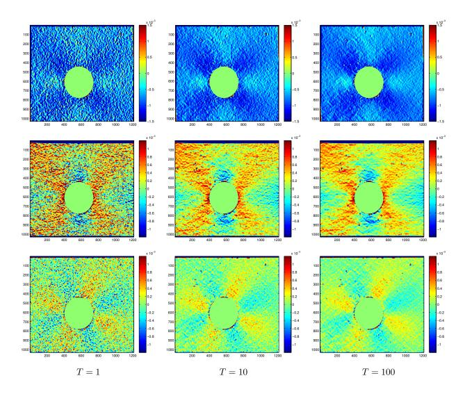
Figure 3: Evolution of the strain components  $\varepsilon_x$  (top),  $\varepsilon_y$  (middle),  $\varepsilon_{xy}$  (bottom) estimated on the averaged grid obtained from  $T = \{1, 10, 100\}$  images. (T = 1 corresponds to a raw image, without any averaging.) The x- and y- axis are respectively the vertical and horizontal axis. Each pixel represents a surface whose area is  $40 \times 40$  micrometers<sup>2</sup> on the specimen.
