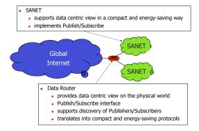
**Fig. 1** Vision of the Internet of Sensors—integration of SANETs within the Internet.
