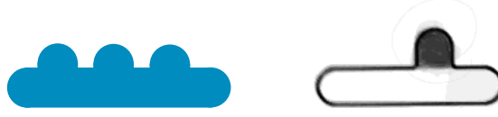
Fig. 9 Shapes with features (bumps) of the same radius as the main shape. The radius of the medial axis transform is nearly constant throughout the shape: the bumps will thus not be detected as salient features using the classical SAT. However, in such cases, the user study clearly indicates that the bump should still be identified as a feature, even without repetition.
