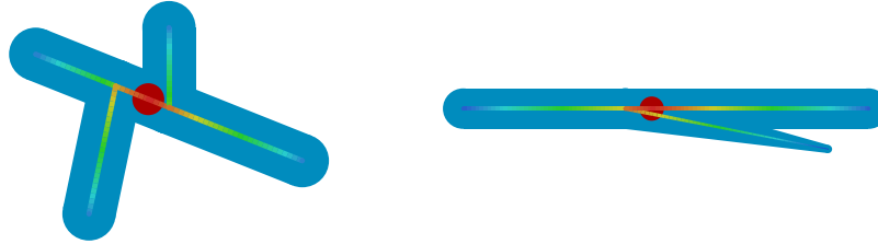
Fig. 10 The medial axis of two shapes, the EDF along the medial axis (in color), and the EMA (red dot).
