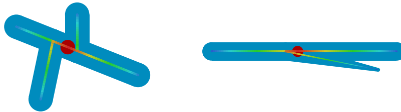
Fig. 10 The medial axis of two shapes, the EDF along the medial axis (in color), and the EMA (red dot).
