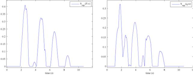
Fig. 12. Repulsive force  $S_{rep}(\mathbf{P}, \mathbf{v})$  and  $S_{rep}(\theta, \omega)$  with both  $S_{rep}(\theta, \omega)$  and  $S_{rep}(\mathbf{P}, \mathbf{v})$
