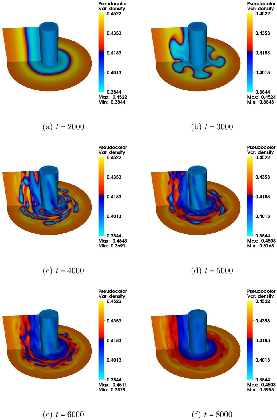
FIGURE 11. Evolution of ion turbulence. The distribution function is shown for the velocity  $v_{\parallel} = 0$ . The mesh size is  $n_x = n_y = 128, n_z = 32, n_v = 65$ . Mixed Semi-Lagrangian/finite difference method is used.
