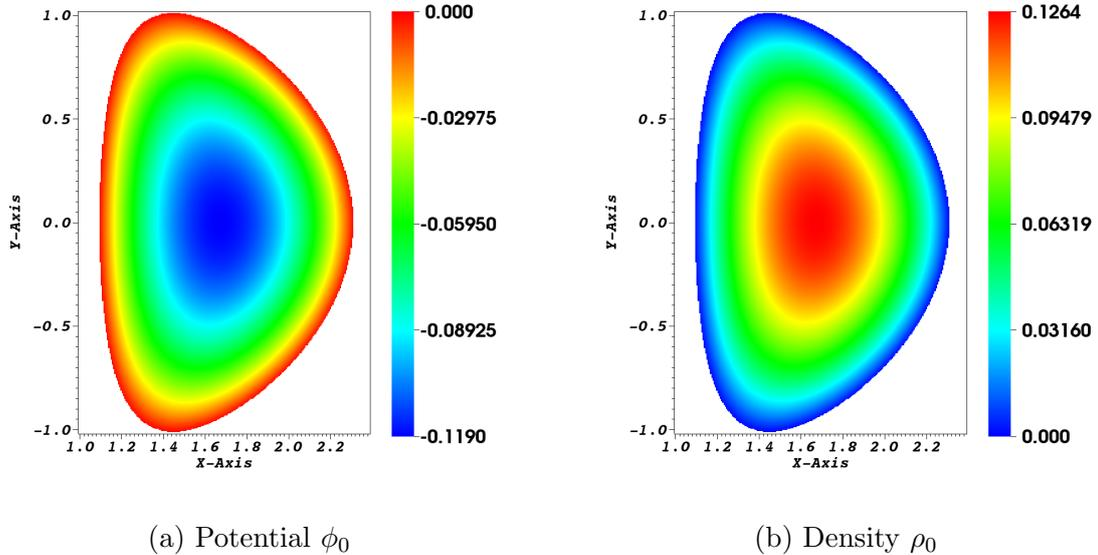
FIGURE 3. A steady state solution of the guiding-center model (2.9) in D-shaped domain. Mesh size is  $n_x \times n_y = 240 \times 440$ .
