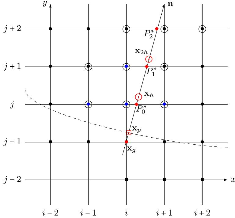
FIGURE 1. Spatially two-dimensional Cartesian mesh.  $\bullet$  is interior point,  $\blacksquare$  is ghost point,  $\square$  is the point at the boundary,  $\circ$  is the point for extrapolation, the dashed line is the boundary.
