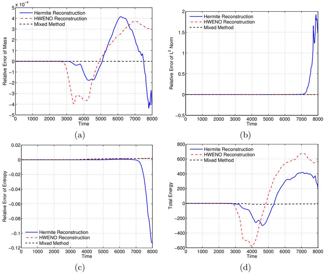
FIGURE 7. Comparison of different reconstruction methods for the conservation laws for the Drift-Kinetic model. The mesh size is  $n_x \times n_y \times n_z \times n_v = 128 \times 128 \times 32 \times 65$ .
