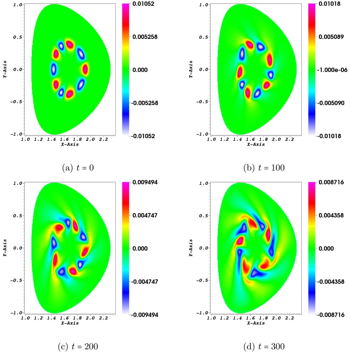
FIGURE 6. Instability simulation for guiding-center model in D-shaped domain. The difference between the perturbed density and the steady state density is presented, *i.e.*  $\delta\rho(t) = \bar{\rho}(t) - \bar{\rho}_0$ .
