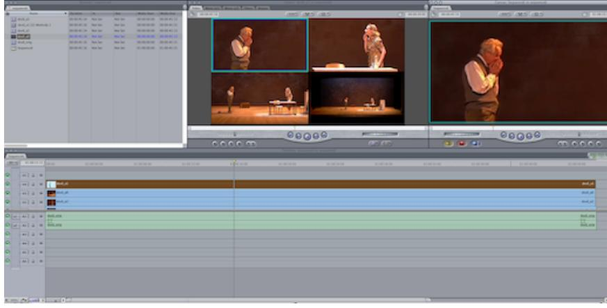
**Figure 7: Screenshot of a multiclip sequence generated using a set of four sequences in Final Cut Pro. In the middle we see the four sequences including the original master shot and three reframed sequences (MS A, MS B, FS All) which were generated using the proposed method. On the right, we see the edited sequence.**
