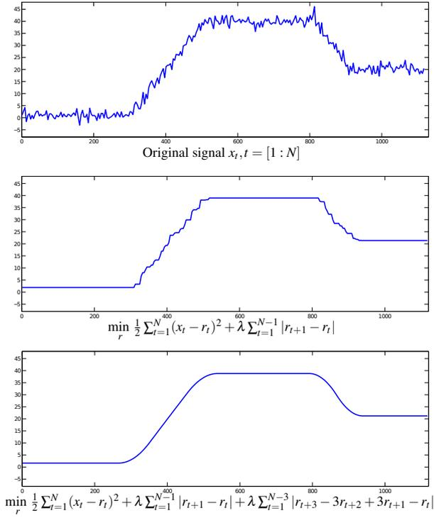
**Figure 6: Top: Synthetic one dimensional data  $x$ . Middle: Optimized signal  $r$ , minimizing the sum of squares closeness term to original data with L1-norm regularization on velocity. Bottom: Optimized signal  $r$ , minimizing the sum of squares closeness term to original data with L1-norm regularization on both velocity and jerk.**
