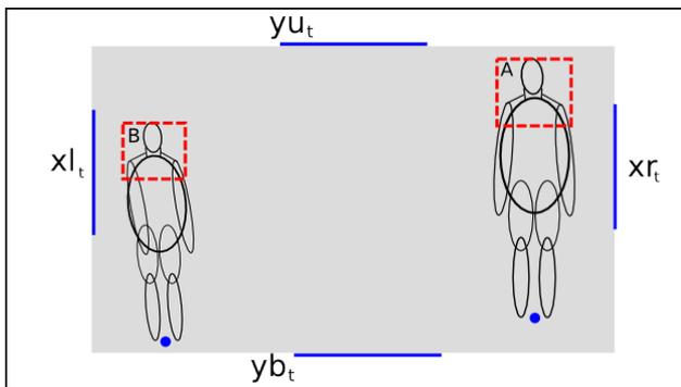
**Figure 4:** Inclusion region for shot specification "FS A,B" i.e. the full shot of Actor A and Actor B. A full shot of two actors is a tightest window which keeps both of them entirely inside the frame.
