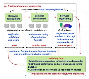
Fig. 1. (a) traditional computer engineering versus (b) our new collaborative performance and cost-aware software/hardware co-design as a web service.
