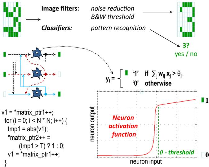
Fig. 2. Conceptual example of pattern recognition, image filtering and character noise reduction using Hopfield fully interconnected and recurrent neural network. Simple C kernel is a part of a neuron activation function processing thresholds for all neurons.
