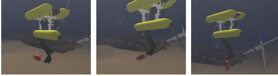
(a) End of approach. The hook is lying on the seabed and the arm cannot follow its setpoint. (b) Beginning of lifting. One of the vertical thruster is saturating. (c) Recovery complete.
