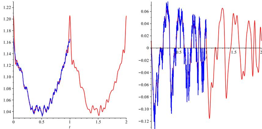
FIGURE 7. For both functions  $\varphi_{2/3}(t)$  (left) and  $\varphi_{1/3}(t)$  (right) from Example 12, their graph computed by the cascade algorithm (between 0 and 1) and by the partial sum of their Fourier series with twenty harmonics (between 0 and 2).
