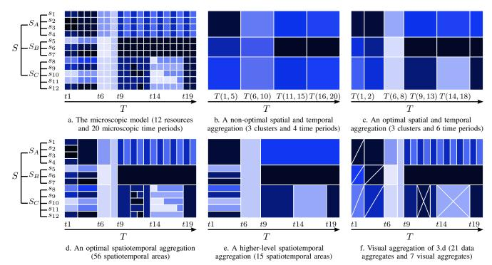
Figure 3. Aggregation and visualization of an artificial trace giving the behavior of 12 resources during 20 microscopic time periods (two possible states)
