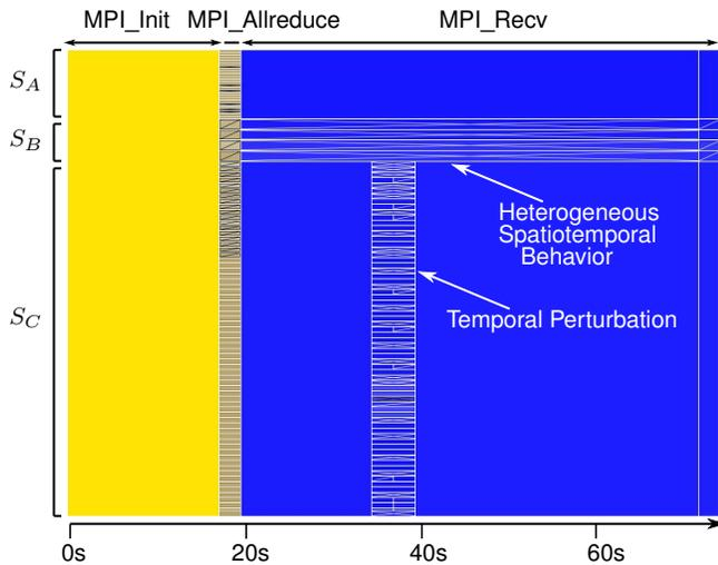
Figure 4. Ocelotl overview of the MPI application LU, class C, 700 processes, executed on the Nancy site of Grid’5000 ( $S_A$ : Graphene,  $S_B$ : Graphite,  $S_C$ : Griffon). We mainly distinguish an initialization sequence (0-20s), followed by the computation phase, where the behavior of the Graphite cluster is heterogeneous in space and time, and there is a perturbation that touches only the execution of the Griffon cluster (34.5s).
