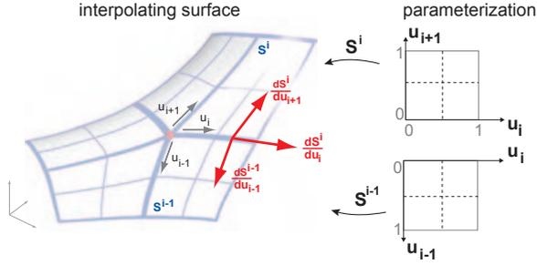
**Figure 3:** 4-split of the parameter domain. Parameterization of the surface patches around a mesh vertex. Always four Bézier patches are constructed in correspondence to each mesh face, called macro-patch. The benefits of the 4-split are mainly that the resulting surface is local and of low degree while interpolating the mesh vertices.
