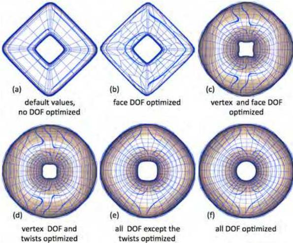
**Figure 8:** Optimization of different subsets of degrees of freedom. All remaining DOF are set with default values. The optimized subsets of DOF are respectively from left to right: (a) no DOF optimized, (b) face DOF, (c) vertex and face DOF, (d) vertex DOF and twists, (e) all DOF without twists, (f) all DOF. The input mesh is the torus mesh of Figure 10, second row. The Bézier control net and isophotes are drawn in blue.
