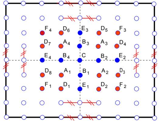
**Figure 7:** Bézier control points of a piecewise bi-quartic macro-patch. The empty control points ensure  $G^1$ -continuity between adjacent macro-patches. The colored control points ensure  $C^1$ -continuity inside a macro-patch.
