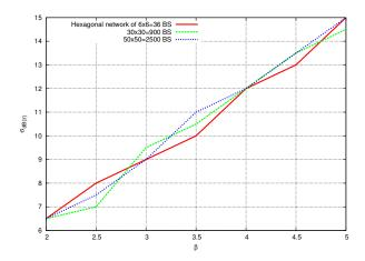
Fig. 1. Critical values of  $\sigma_{dB}$  in function of the path-loss exponent  $\beta$ , for different network sizes, above which, the empirical distribution of  $L^*$  in the hexagonal network cannot be distinguished from this for the "equivalent" Poisson model at a 99% confidence level, for 9/10 realizations of the hexagonal network.
