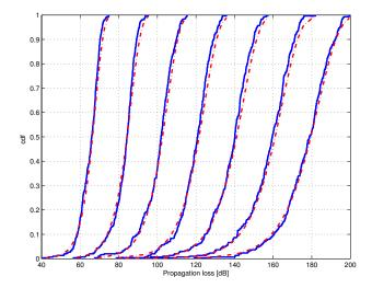
Fig. 2. Visual comparison of the empirical distribution of  $L^*$  in the hexagonal network of  $6 \times 6 = 36$  base stations (solid lines) to the theoretical cdf of  $L^*$  in the "equivalent" Poisson model (dashed lines) for  $\beta = 2, 2.5, 3, \ldots, 5$  (curves from left to right) and the corresponding critical values of  $\sigma_{\rm dB} = \sigma_{\rm dB}(\beta)$  taken from Figure 1.
