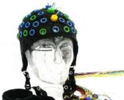
Figure 12: Cap with 64 endowed positions of electrodes according to the international system
