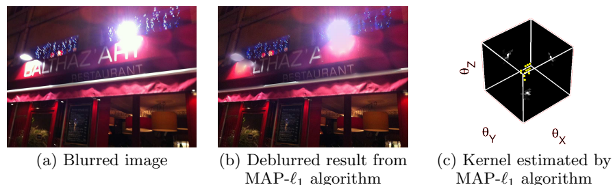
Figure 1.8 Blind deblurring failures. A blurred image (a) with the deblurred result (b) and kernel (c) estimated by the MAP- \ell_1 algorithm. This image contains a large amount of noise, and was captured with a camera-phone whose response function is unknown. As a result, the algorithm fails to estimate a good kernel, and instead returns a kernel which is close to a delta function.
