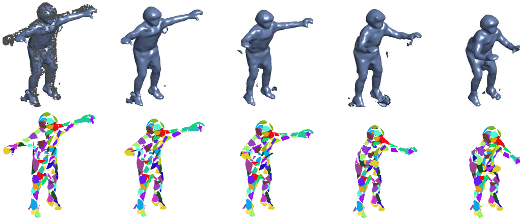
Figure 4. 3D point registration using the proposed approach: ( top ) the MPU interfaces describing different frames 44, 47, 49, 55, 75; ( bottom ) the deformed source patches.
