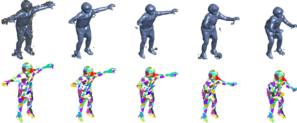
Figure 4. 3D point registration using the proposed approach: ( top ) the MPU interfaces describing different frames 44, 47, 49, 55, 75; ( bottom ) the deformed source patches.
