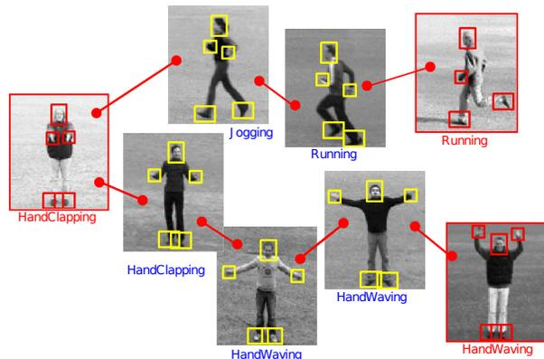
**Fig. 1.** Joint pose estimation and action recognition in the image graph. Training images (red frames) are manually annotated with the position of body parts and action labels. Part positions and action labels in test images (yellow frames) are resolved by optimizing the global graph energy.
