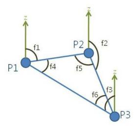
Fig. 6. Diagram explaining the 3D invariant construction. The 3 points described ( $P_1$  to  $P_3$ ) and their triangle are in blue.  $f_1$  to  $f_6$  are the angles used as features. The 3 vertical green arrows represent the vertical axis.
