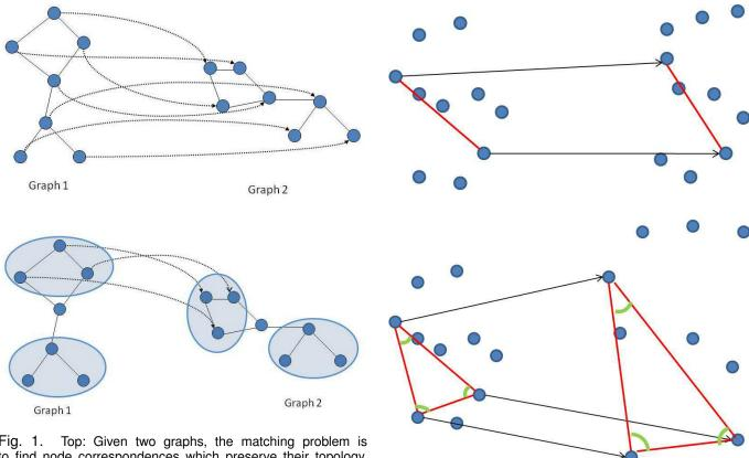
Fig. 1. Top: Given two graphs, the matching problem is to find node correspondences which preserve their topology. Bottom: In a hypergraph, one hyperedge can link more than 2 nodes. As an example, in this figure four hyper-edges are represented by circles. Each of them regroups 3 nodes that they link together. The three matches drawn on the bottom figures induce a matching between two hyperedges.
