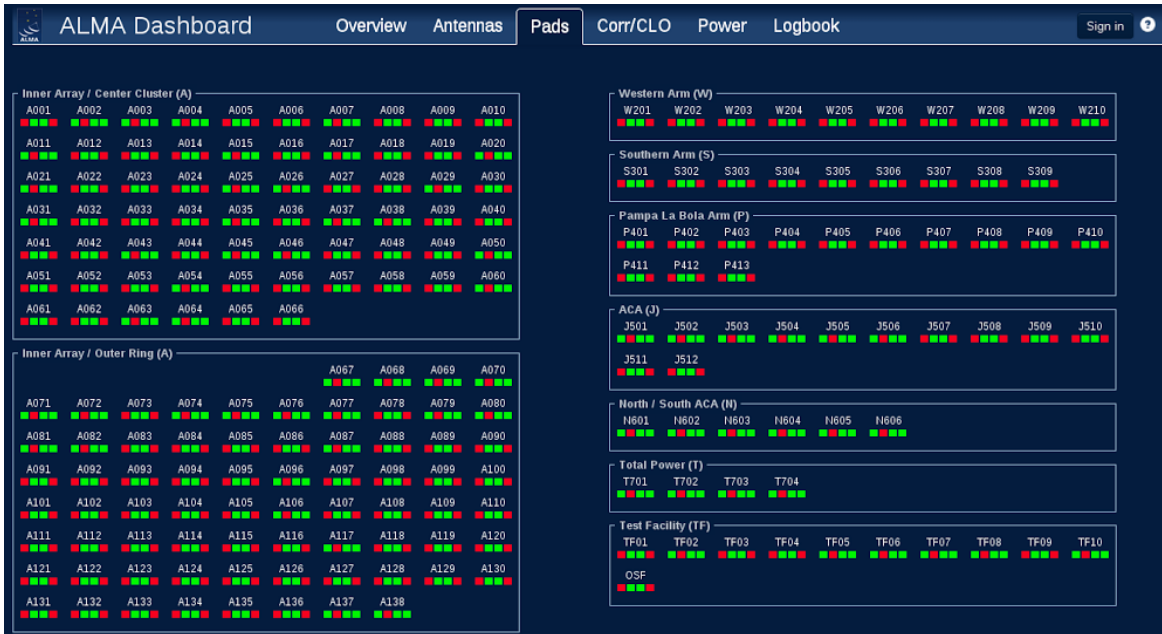
Figure 12. Mockup of the Pads tab. Pads are grouped by geographical area. Four substates are associated with each one of them, and can be toggled by simple clicks on the corresponding colored square: accessibility of pad to ground vehicles, signal vault, power vault, ridges and structure.
