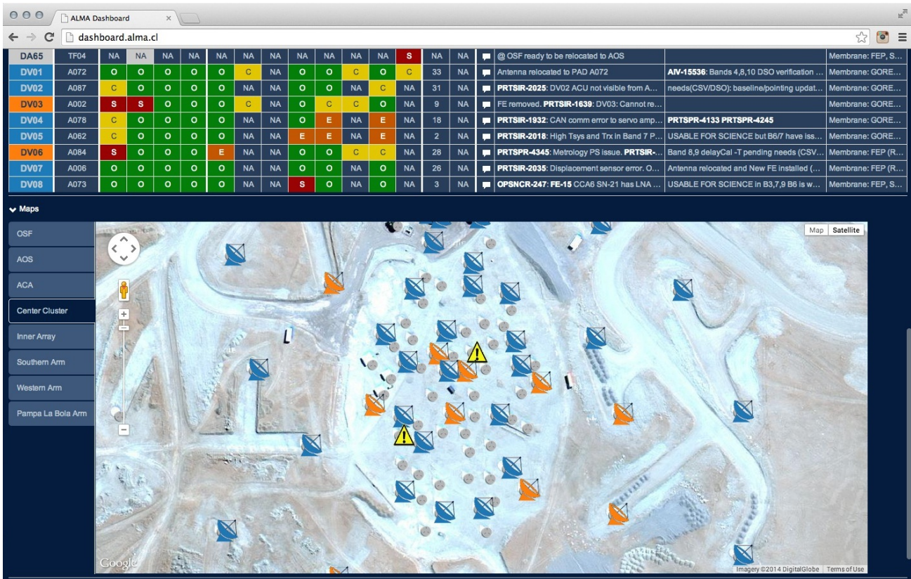
Figure 5. Representation of antennas showing their geographical location using a Google Map widget. Tabs on the left-hand side of the map act as navigation shortcuts to center and zoom the map on a particular area of ALMA.
