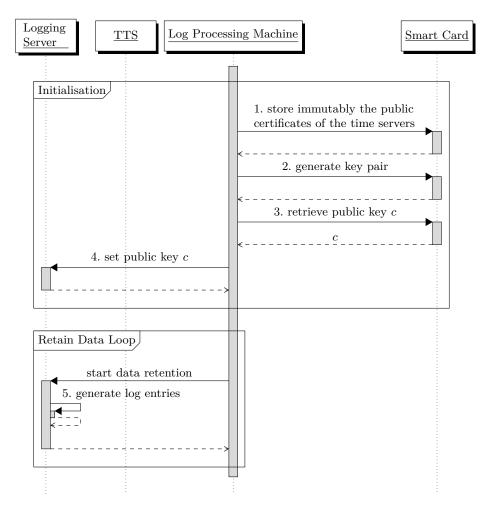
${\bf Fig. 1. } Logical steps of the data retention compliant logging-initialisation and logging.$
